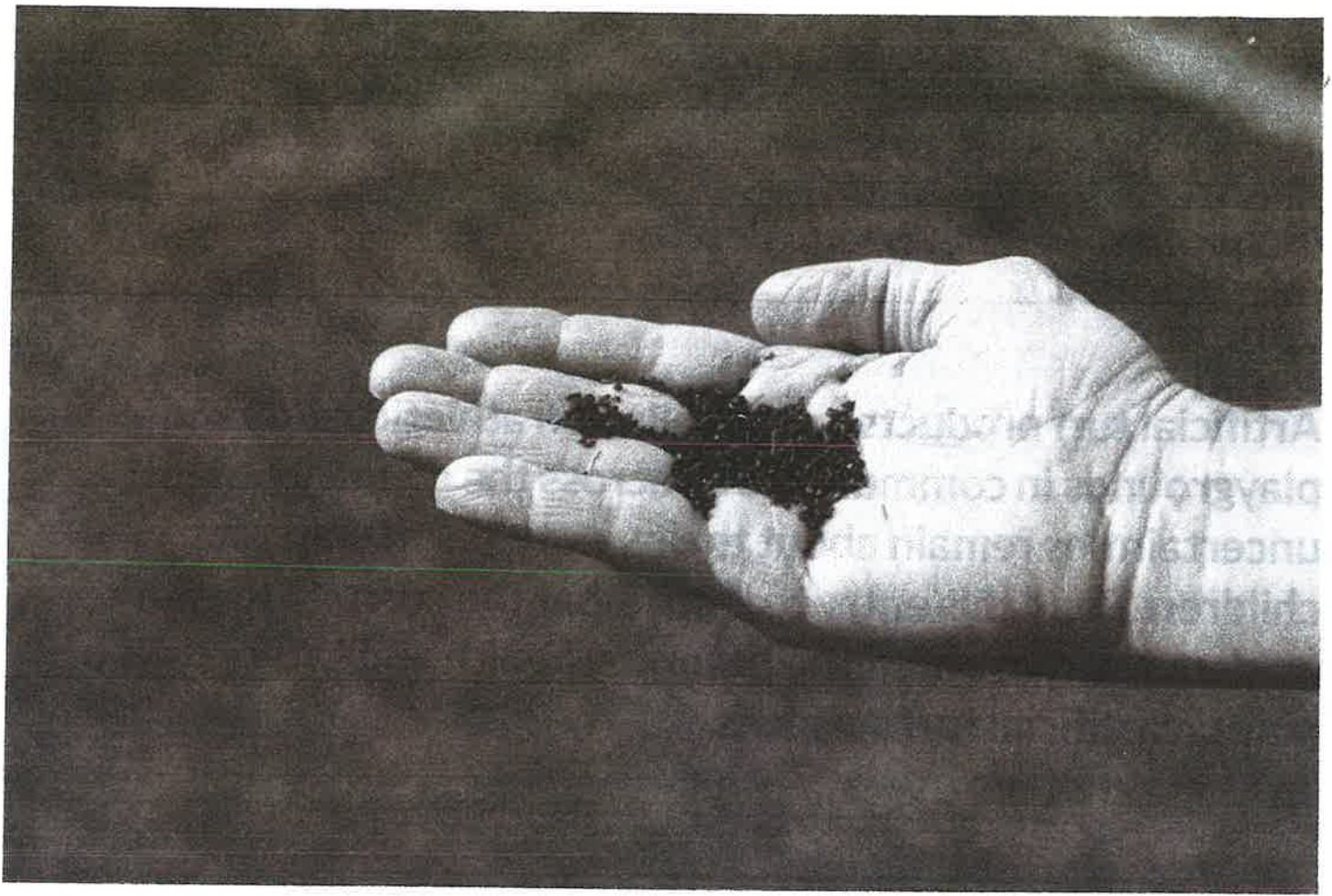
Close-up: rubber infill that provides cushioning and serve as a base for the blades.
