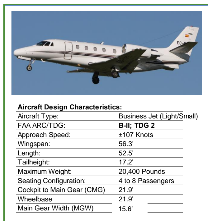
Figure 3-1: Cessna Citation XLS Characteristics
