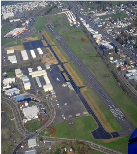
After many years of environmental study, design and preparation, the project to move the parallel taxiway at the Roseburg Regional Airport is substantially complete. The \$4.88 million construction phase was completed in December. The only remaining item, a second coat of striping, will be finished during warmer weather next summer.
